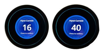
The Breaker Setting should be set at **16** if your **ECO SPA** was set at the factory for **110 Volt** operation.
